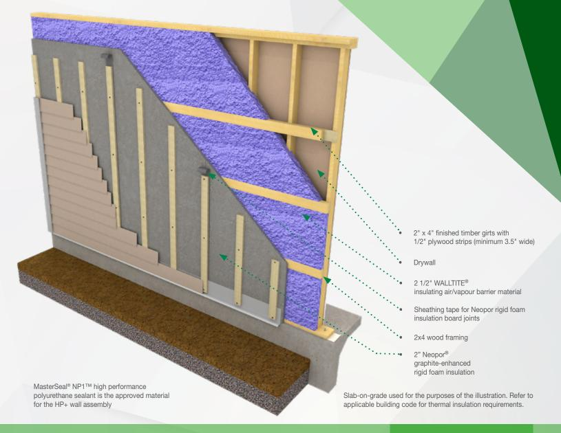
HP+ Wall System XR Series is a strong structural assembly that meets or exceeds building code requirements with a minimum nominal insulation R-value of R-25.2 up to R-45.8 with 2x4 wood framing. The XR Series offers exceptional energy and cost efficiencies.
